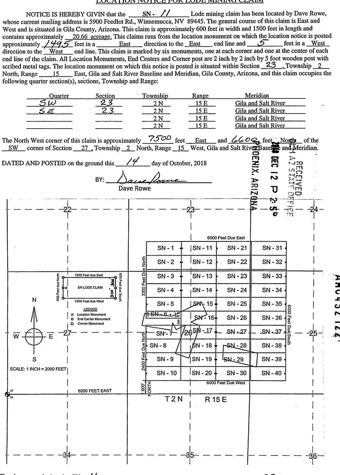
The above map depicts the SN-Lode mining claim, which is located in Section(s) North, Range 15 East. Gila and Salt River Baseline and Meridian, Gila County, Arizona. The claim corners, end centers and Location monuments are marked by 2 inch by 2 inch by 5 foot wooden post with aluminum tags. The bearings and distances between claims and tie point are depicted on the map.
